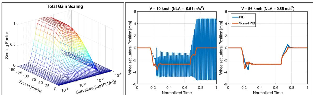
Figure 1 - Gain Scaling function (Left), application of Gain Scaling on wheelset control (Right)
