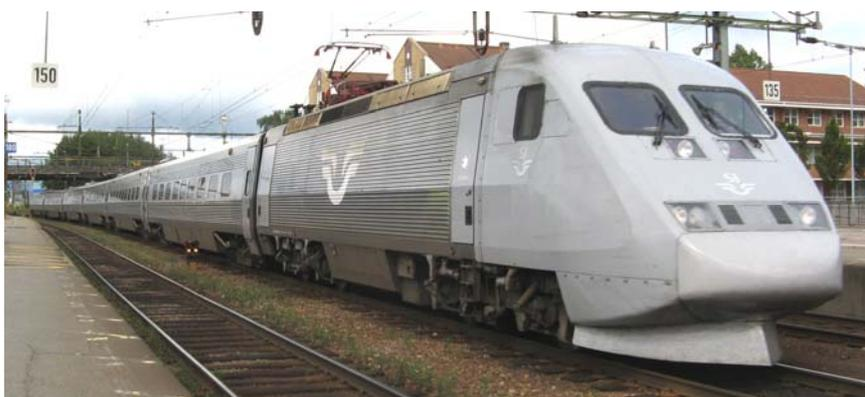
**Figure 2** *X 2000* high-speed tilting train, operated by *SJ AB*
