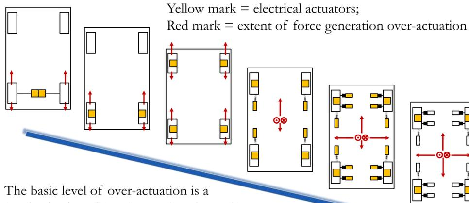
The basic level of over-actuation is a longitudinal model with two electric machines mounted in the center of the rear axle. More actuators will be added in longitudinal, vertical and lateral direction in the following stages until a fully over-actuated corner module. The main advantages of this approach are the focusing on single subsystems, the heritage of developed solutions and proximity to series application in the vehicle industry.
